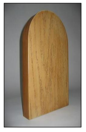
Material is factory primed with beige primer. To obtain the wood look, the door must be stained in a two color process by a professional painter.  Apply a dark stain first to go into the "grain." This is wiped off the flat part of the steel.
