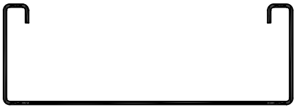
Case Open w/ Drywall Returns
