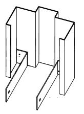
Strap Anchors into Throat Standard for Wood Stud and Compression Anchors
